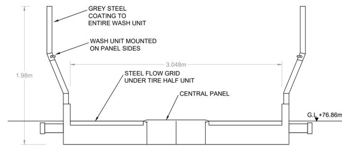
**ELEVATION OF UNIT FROM TRUCK MOUNTING SIDE**
