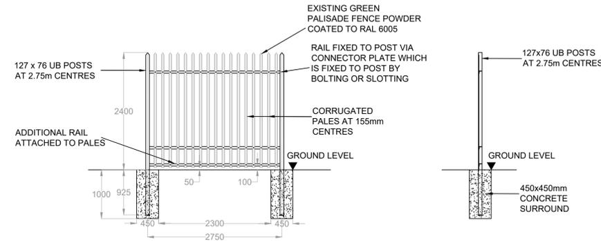
**TYPICAL DETAIL OF PALISADE FENCING (TYPE 3)**
